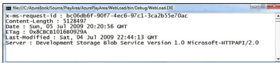
Figure 9.8 The output of a HEAD request
