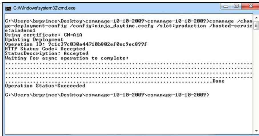
Figure 18.14 We've uploaded a new configuration file for our service. Because we changed only the number of instances for each role, we didn't have any downtime. The FC has spun up new instances to meet our needs.
